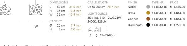
STANDARD The fixture is supplied with lamps. Black canopy with cover plate in matching colour of the fixture. Leading edge dimmable.
